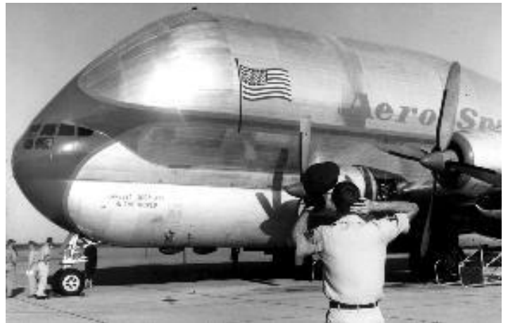
The "Pregnant Guppy" – a converted C-97 designed to transport the Saturn launch vehicle for NASA
