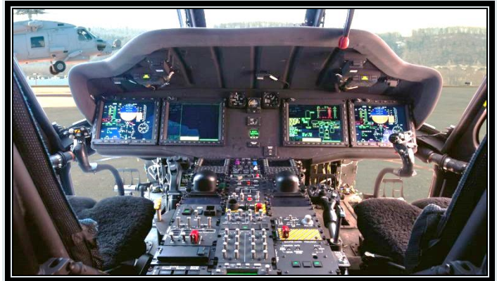
The Lockheed Martin Common Cockpit™ avionics suite is common to the U.S. Navy's MH-60R and MH-60S multi-mission SEAHAWK helicopters.
