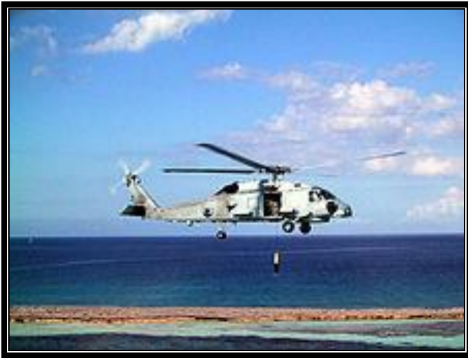
An MH-60R Seahawk conducts sonar operations.
