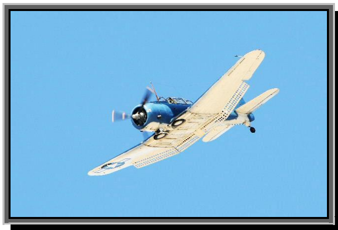
The Planes of Fame's Douglas SBD Dauntless, showing her air brakes, which allowed this venerable dive bomber to dive straight down on the target, then brake the dive and pull up away from the blast. SBDs were crucial in victory at the Battle of Midway.
